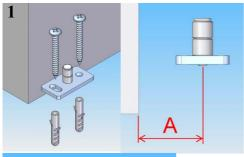
Before installing the door guide, first checking the door thickness for determining distance "A" (center of door guide to wall) according to the wooden door installation instruction dimension, then drilling appropriate holes on the ground, inserting suitable anchors then tightening screws to fix the door guide. If the rail frame is screwed to the ceiling, distance "A" is measuring from the center of door guides to the outside edge of rail frame
