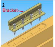
Checking page 1 of wooden door installation instruction for wooden door cutout, and make the appropriate cutout on the top of wooden door for the bracket, then fixing the bracket to wooden door with 4 tapping screws, one bracket each side left and right hand of wooden door.
